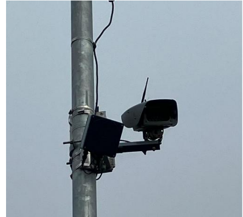
A noise camera made by the company Jenoptik, pictured during a trial in Exmouth
